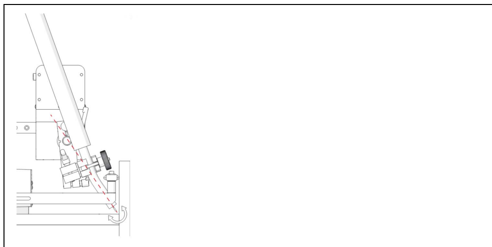
Fig. 10 Adjusting the welding torch
